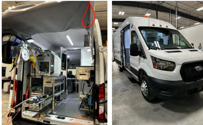
Typical Sewer Camera Truck
